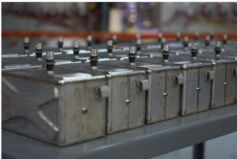
Ambri's batteries require temperatures of around 750 to 1,000 degrees Fahrenheit to operate.
